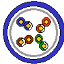
Screened Unshielded Twisted Pair (S/UTP, F/UTP, or SF/UTP) (a.k.a. FTP)
